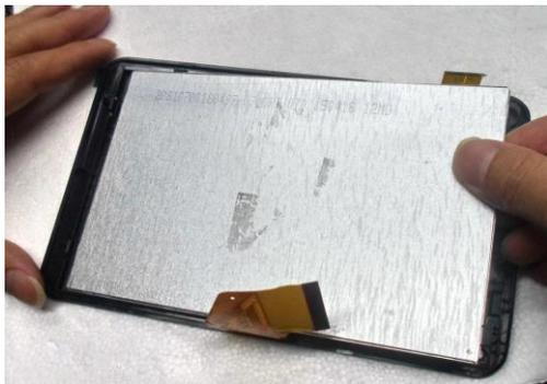
3. After releasing the button mechanism, carefully extract the LCD
